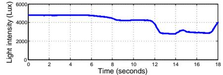
**Figure 5. Light intensity during the rotation in the outdoor environment.**
