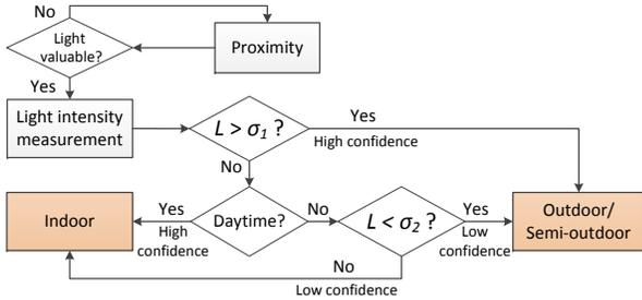
Figure 6. Detection flow of light detector.
