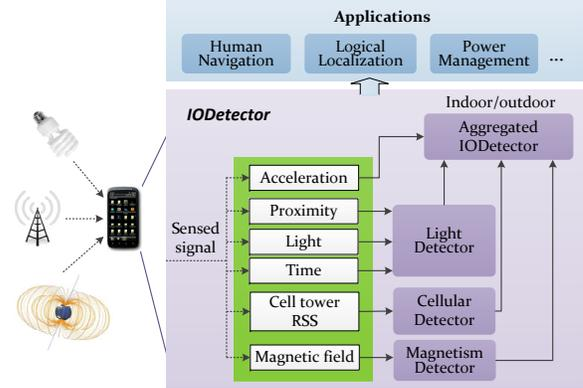
**Figure 2. System architecture of IODetector.**
